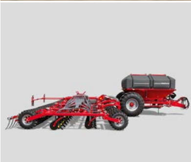
Sprinter 12 SW: Support wheel with intermediate packer
