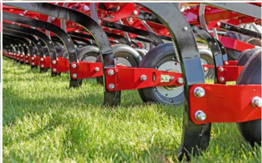
NT chisel coulters remove lumps from the seed horizon and place the grain precisely
