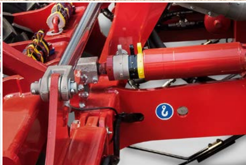
Individual depth adjustment with ClipOn spacers
