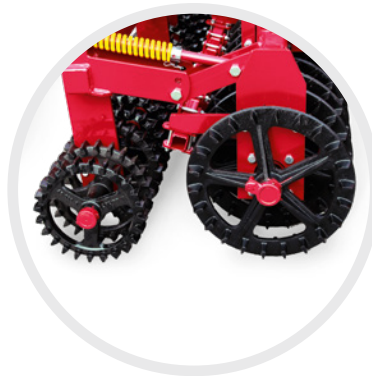
Crosskill roller in combination with Crosskilette for demanding, heavy soils for even better re-compacting of the soil
