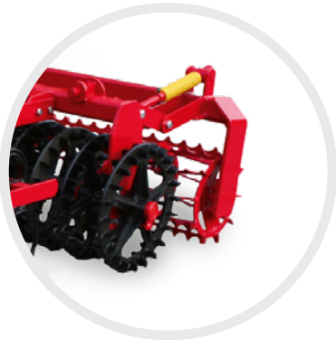
Centrally placed Crosskill component for a better crumb structure and better re-compacting of the soil
