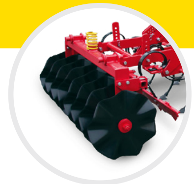
Corrugated discs at the front so that heavy vegetation can be cut
