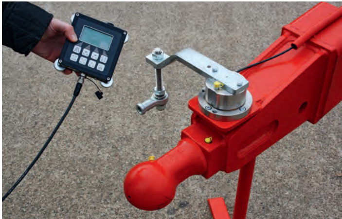
The electronic forced steering system allows operators to select one of many programs that control the trailer's response to their steering.
