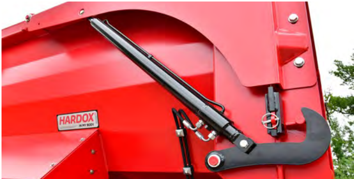
Better seal of the tailgate trough locking hooks and a lock-pressure valve.
