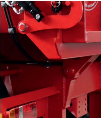
Massive tipping bearings with one full-length 40 mm pin are used on the SK trailers. This gap-free assembly has not failed a single time in more than 30 years.
