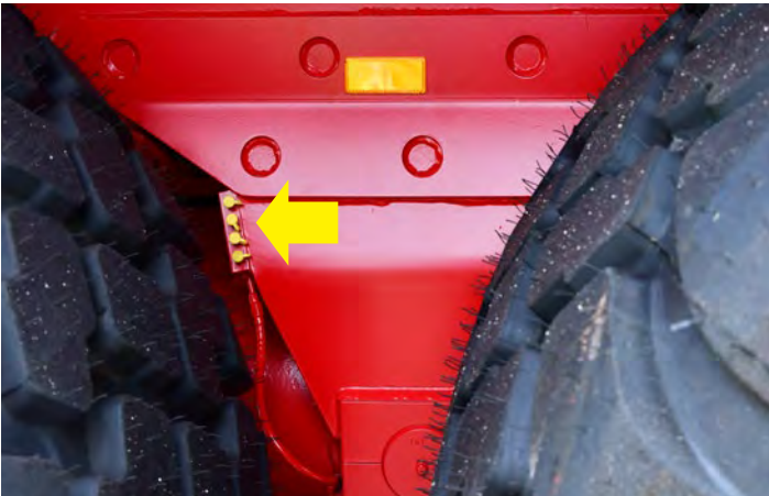
Machines with walking beam running gear or independent hydraulic wheel suspension have a lubrication bank that attends to all greasing points, especially those in awkward positions.
