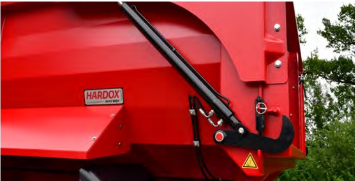
For the transport of coarse grained and stones, the locking hooks remain in open position by turning the locking pieces.
