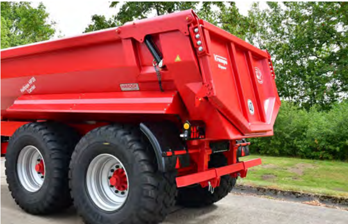
Option: The underride guard swings up to give optimum ground clearance in difficult terrain.
