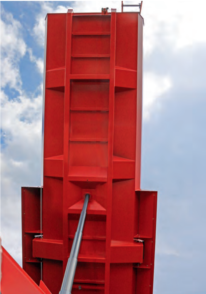
The base of the floor on the SK models is heavily ribbed for superior rigidity of the structure. The base bearers are made from section steel rather than from cheap angle bars. The braces underneath the body are fully welded to eliminate any cavities and risk of corrosion.
