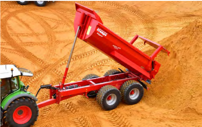
The Tandem HP 20 Halfpipe is an earthmoving tipper for real professionals and complies with commercial approval legislation, hence requiring no special permit for travelling on public roads in Germany.
