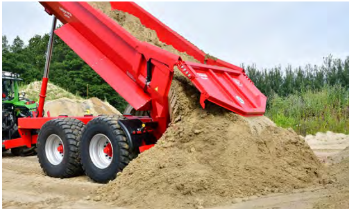
The tailgate pivots open.
