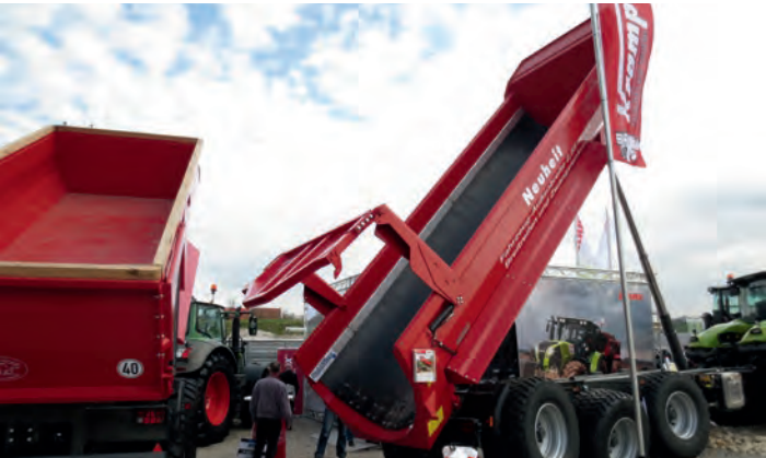
The plastic 'Okuslide' lining for trailer bodies is a retrofit option which ensures the cargo glides off smoothly and quickly, so no material is left in the body (even when working in sub-zero temperatures).
