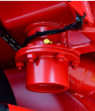
The heavy-duty 80 mm and 100 mm ball bearings on the heavy-duty Tridem tippers and Halfpipe earthmovers have replaceable PU wearing cups.
