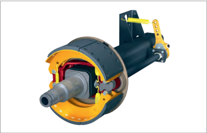
This illustration shows the cross section of a profi axle – generously sized wheel bearings and a massive stub axle.
