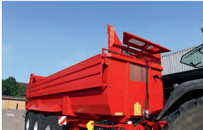
The combination of side- and front-foldable extensions provides increased volume, a variable transfer height, and good visibility. The locking and release of the silage extensions can also be optionally and much more easily operated from below, standing next to the trailer, using a robust lever.
