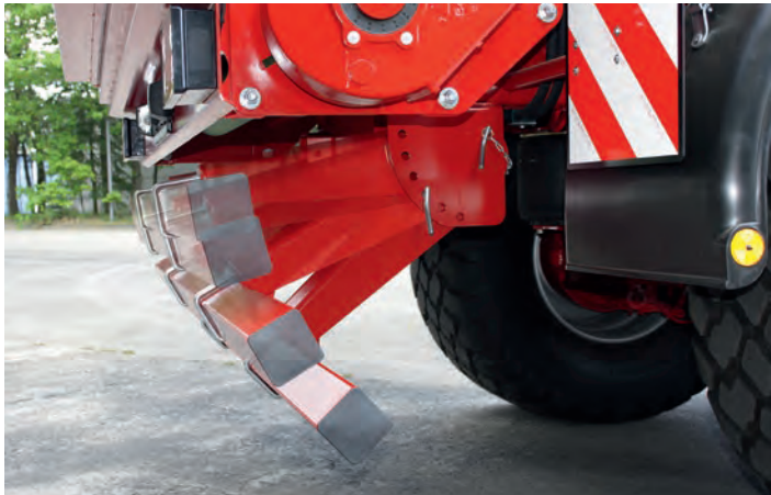
The height of the pivoting underride guard can be adjusted without the use of tools.
