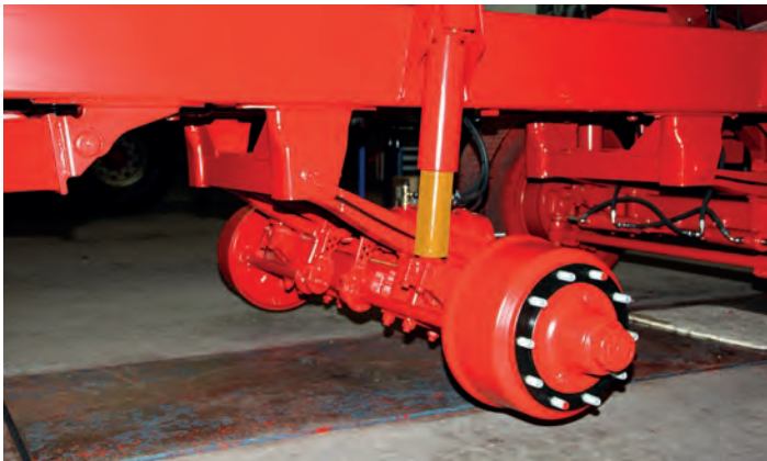
Few manufacturers can match Krampe's experience in building hydraulic running gear. The standard guard tubes protect the chrome-plated piston rods against damage from stones.
