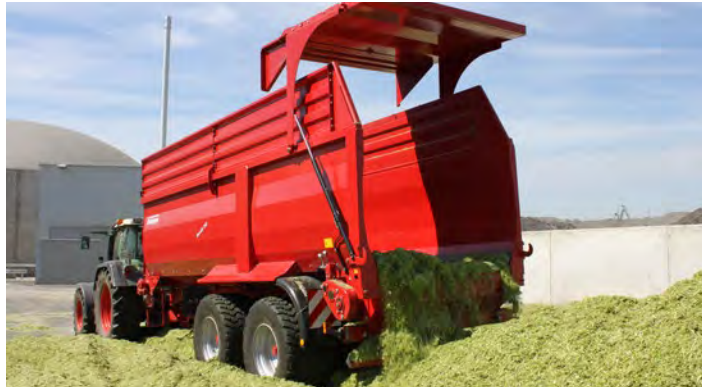
The silage extensions are available as aluminium profiles with a construction height of 40 cm or as steel profiles with a construction height of 60 or 80 cm.
