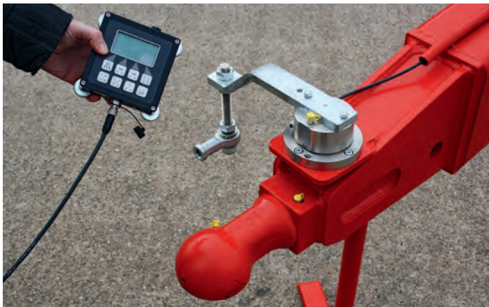
With the electronically controlled forced steering system, the driver can use various modes to control the steering of the trailer.
