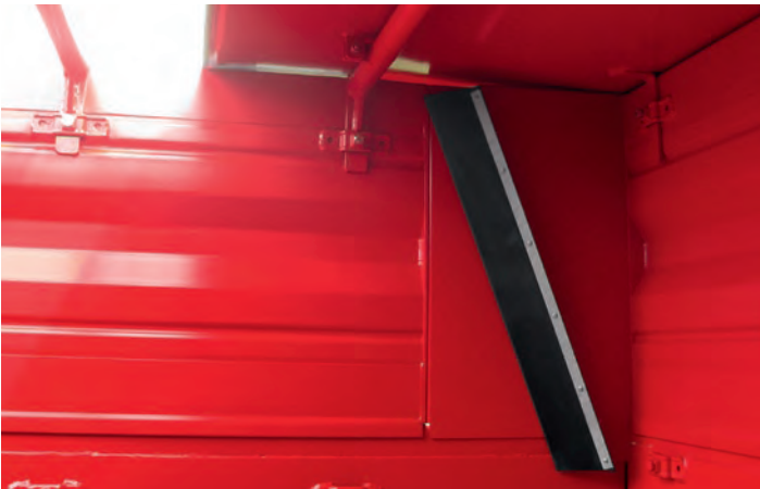
A rubber lip seals the extensions against any loss of grain.
