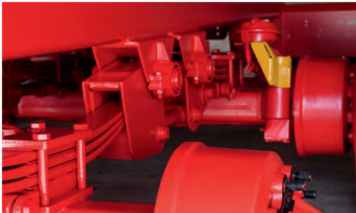
The steering axle with raised cylinder provides absolute ground clearance and keeps the brake cylinders out of the danger zone.
