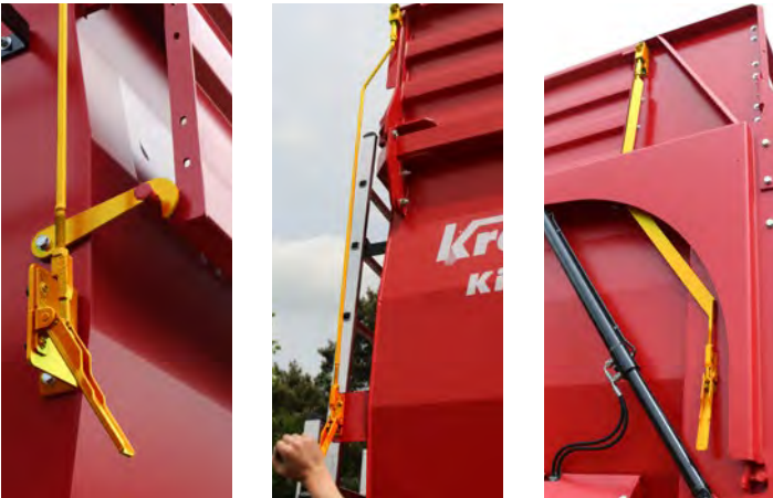
The combination of side- and front-foldable extensions provides increased volume, a variable transfer height, and good visibility. The locking and release of the silage extensions can also be optionally and much more easily operated from below, standing next to the trailer, using a robust lever.
