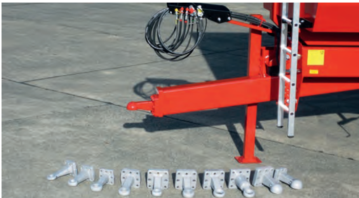
The drawbar can be specified with rubber, air or hydraulic suspension and offers almost infinite y variable height control.
