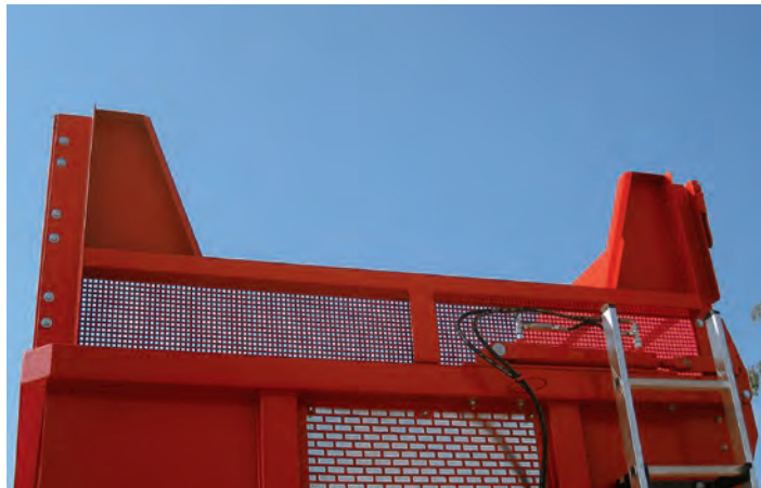
The top of the headboard is V-shaped, offering easier filling when the trailer is following behind the forager.
