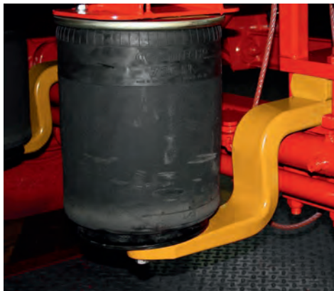
Air suspension with double springs and large pneumatic bellows ensure exceptionally quiet running.
