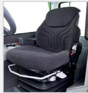
Pneumatic seat for improved comfort.
