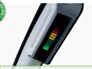
The traffic light indicator on the right side pillar provides a fast and clear information about the machines stability
