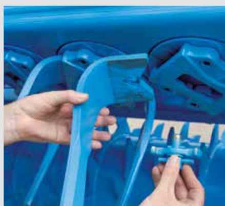
Replacing a quick-change tine
